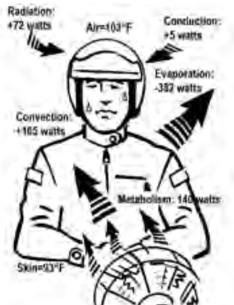
Figure 5 Heat Balance Wearing a Vented-Wind-proof Suit With 103°F Air Temperature Required Evaporation: 19 oz. per hour
