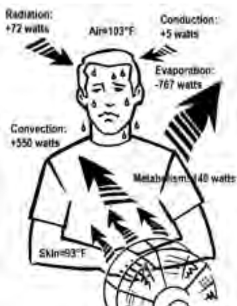
Figure 4 Heat Balance Exposed to High Wind Speed With 103°F Air Temperature Required Evaporation: 39 oz. per hour!
